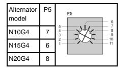
P5 [kVA] limits the maximum excitation voltage of the alternator and therefore the maximum output power of the generator. This parameter is an integral over time, allowing a 200%-300% overload for a few seconds without limiting and illuminating L2 (Red LED blinking 3 times) or a slight overload for a longer period.
