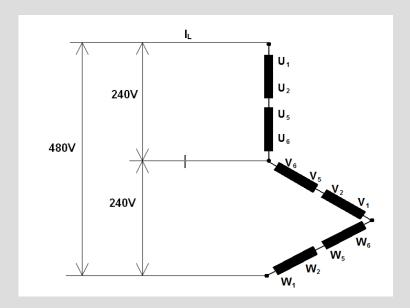
The maximum rating available from Winding 311 in this series zig-zag connection is limited to the following.
