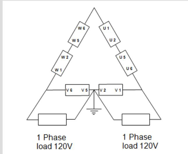
Therefore; as soon as 120V at 100A (12kVA) is being taken from one of the 110V 1-Phase outputs, there is no capability for any 3-Phase output. True, there are the other 120V 1-Phase outputs, which could also provide some 12kVA, but these must remain two individual separate outputs.
