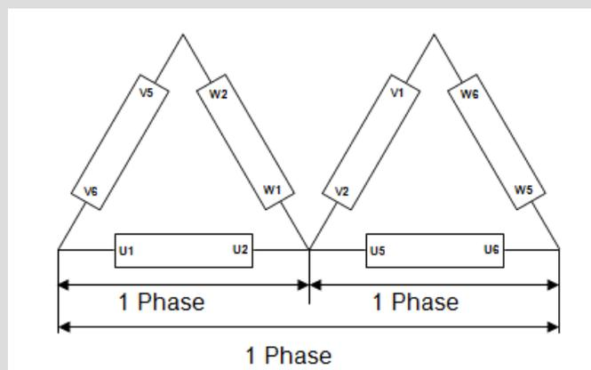
The Double Delta connection is commonly used to utilise a 3-phase winding for a single phase output. This reconnection provides the possibility of a mix of 240V and 120V outputs simultaneously, but the current through the bottom leg when 240V and 120V are being taken, must not exceed the total current of 200A ( $48kVA / 240V$ ). In effect, the Double Delta connection gives a 4 wire single phase system. Windings 1 – 5 and 2 – 6 can be paralleled to give the full 48kVA (200A) at 120V.
