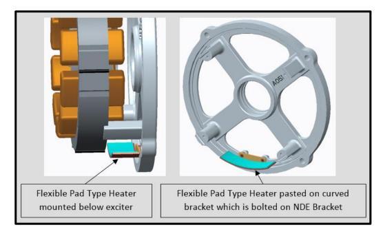
Heater options for the S0L1 are (Drawing A12-H11):
