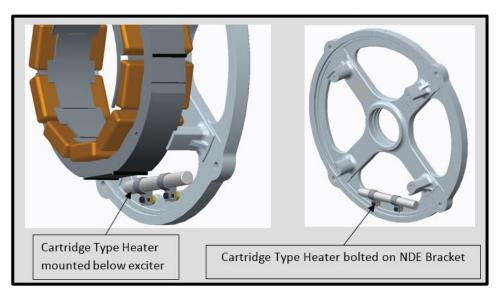
Heater options for the S1L2 are (Drawing A12-H11):
