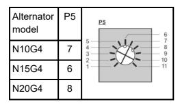
P5 [kVA] limits the maximum excitation voltage of the alternator and therefore the maximum output power of the generator. This parameter is an integral over time, allowing a 200%-300% overload for a few seconds without limiting and illuminating L2 (Red LED blinking 3 times) or a slight overload for a longer period.
