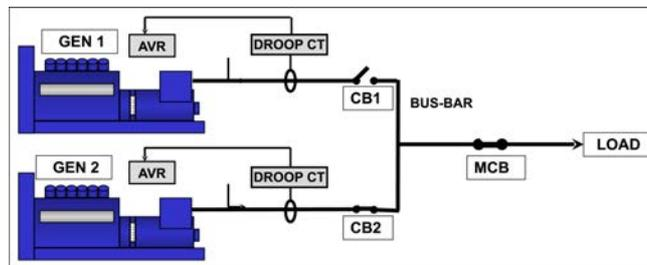
FIGURE 6. ALTERNATEURS PARALLÈLES OU DE SYNCHRONISATION
