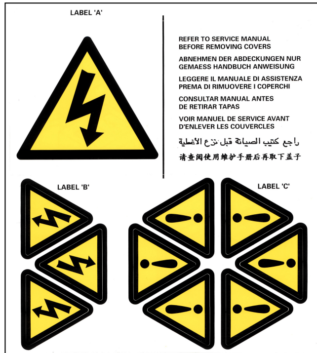
FIGURE 2. HAZARD WARNING LABELS
