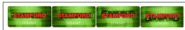
FIGURE 13. DOTS VISIBLE IN LEFT, RIGHT, UPPER AND LOWER VIEWS OF 3D HOLOGRAM
