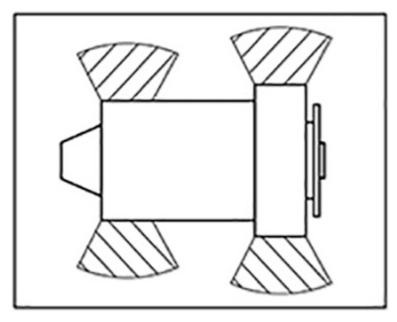
FIGURE 5. S0/S1 ALTERNATOR HAZARD ZONES
