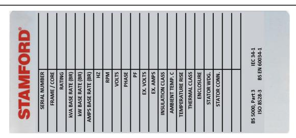
FIGURE 14. GLOBAL STAMFORD AC ALTERNATOR RATING PLATE
