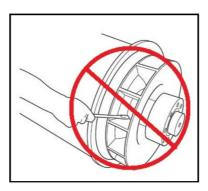
FIGURE 19. DO NOT ROTATE WITH A LEVER
