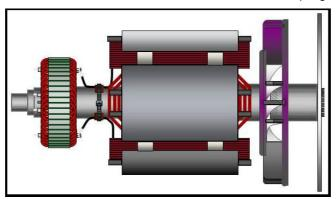
FIGURE 20. SINGLE BEARING ALTERNATOR ROTOR SHOWING COUPLING DISCS BOLTED TO DRIVE END COUPLING HUB (AT RIGHT)
