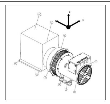
FIGURE 17. VIBRATION MEASUREMENT POSITIONS
