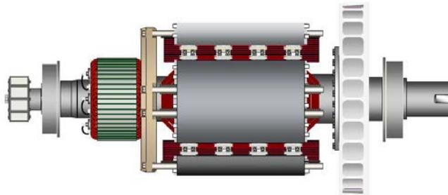
**FIGURA 21. ROTORE DELL'ALTERNATORE A DUE CUSCINETTI CON ALBERO CON CHIAVETTA PER ACCOPIAMENTO FLESSIBILE (A DESTRA)**
