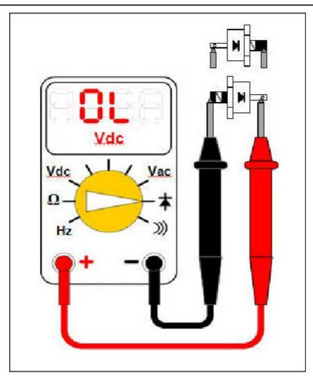
FIGURE 34. DIODE RESISTANCE MEASUREMENT
