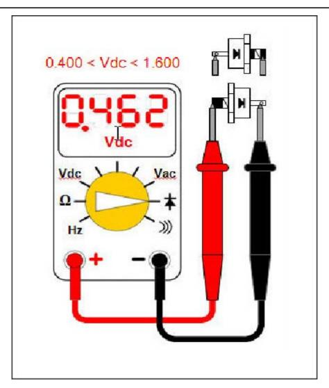
FIGURE 33. DIODE VOLTAGE DROP MEASUREMENT
