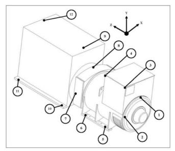
FIGURE 18. VIBRATION MEASUREMENT LOCATIONS
