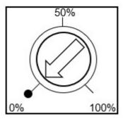
FIGURE 26. AVR [VOLTS] CONTROL POTENTIOMETER 0%
