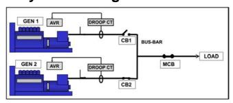
FIGURE 23. PARALLEL OR SYNCHRONIZING ALTERNATORS
