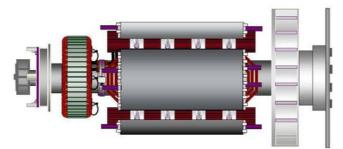
FIGURE 20. SINGLE BEARING ALTERNATOR ROTOR SHOWING COUPLING DISCS BOLTED TO DRIVE END COUPLING HUB (AT RIGHT)
