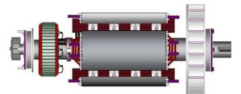
FIGURE 21. TWO BEARING ALTERNATOR ROTOR SHOWING SHAFT WITH KEYWAY FOR FLEXIBLE COUPLING (AT RIGHT)
