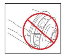
FIGURE 19. DO NOT ROTATE WITH A LEVER
