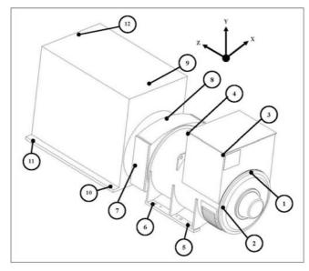
FIGURE 18. VIBRATION MEASUREMENT LOCATIONS
