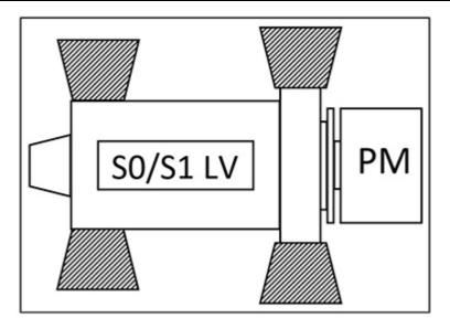
FIGURA 5. ZONE DI PERICOLO DELL'ALTERNATORE S0 E S1
