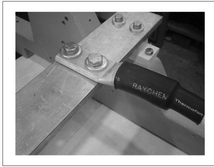
FIGURE 25. CORRECT CABLE CLAMPING
