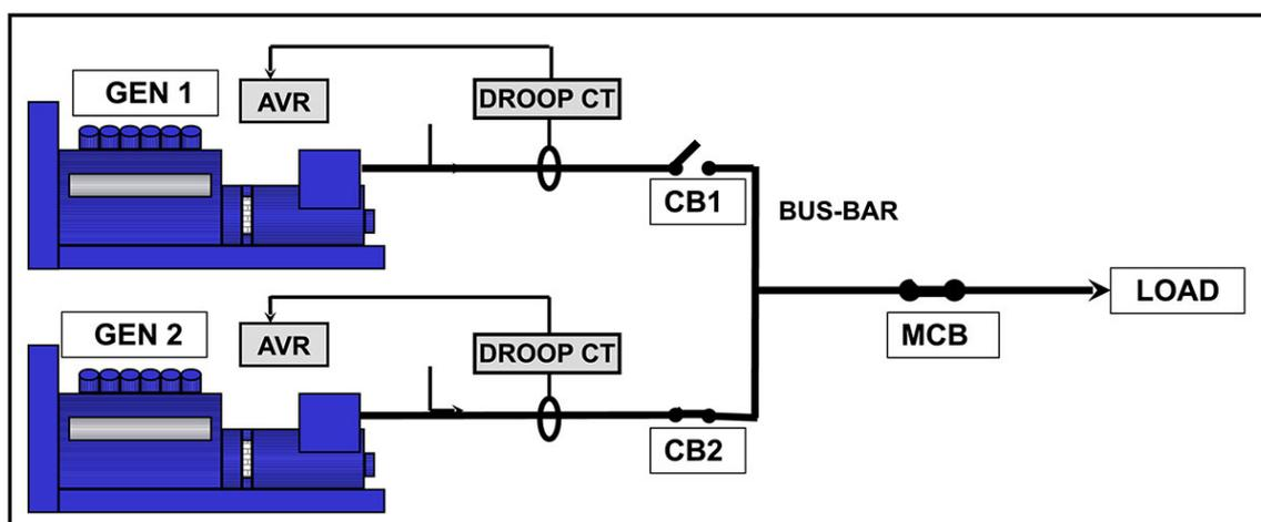
**FIGURE 26. PARALLEL OR SYNCHRONIZING ALTERNATORS**
