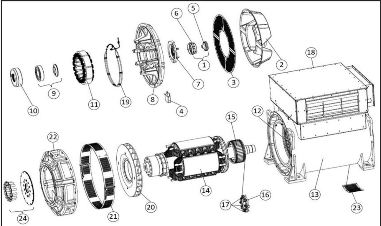
FIGURE 30. S9 LOW VOLTAGE ONE BEARING ALTERNATOR
