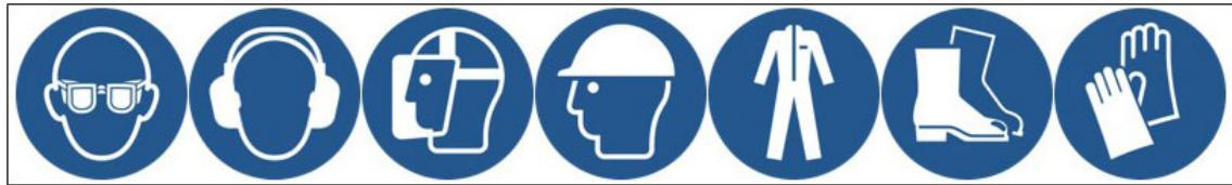
FIGURE 1. MINIMUM RECOMMENDED PERSONAL PROTECTIVE EQUIPMENT (PPE)
