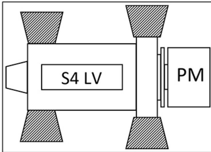
FIGURA 5. ZONE DI PERICOLO DELL'ALTERNATORE A BASSA TENSIONE S4
