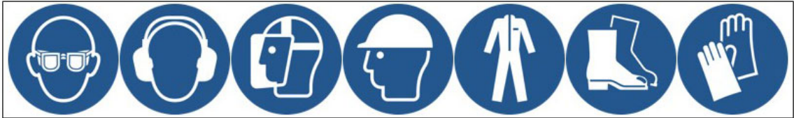
FIGURE 1. MINIMUM RECOMMENDED PERSONAL PROTECTIVE EQUIPMENT (PPE)
