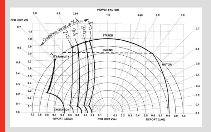
For example; the above Capability Diagram has been created for an alternator rated at 100kVA. From that alternator's technical data sheet, we can read the synchronous reactance (Xd) value is 2.0pu at 100kVA. The load to be considered has been identified as being 70kVA at 0.8 pf lead.
