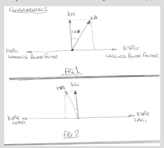
However, if a Generating Set is connected to an electrical network (Mains Grid System), then operational P, Q & S can be adjusted and controlled by functions associated with the Generating Set. Real power P is controlled by the mechanical power (torque) being applied to the Generator's input shaft.
