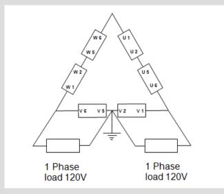
Therefore; as soon as 120V at 100A (12kVA) is being taken from <u>one</u> of the 110V 1-Phase outputs, there is no capability for any 3-Phase output. True, there are the other 120V 1-Phase outputs, which could also provide some 12kVA, but these must remain two individual separate outputs.
