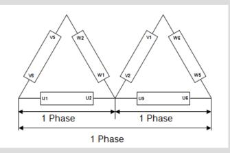
The Double Delta connection is commonly used to utilise a 3-phase winding for a single phase output. This reconnection provides the possibility of a mix of 240V and 120V outputs simultaneously, but the current through the bottom leg when 240V and 120V are being taken, must not exceed the total current of 200A (48kVA / 240V). In effect, the Double Delta connection gives a 4 wire single phase system. Windings 1 - 5 and 2 - 6 can be paralleled to give the full 48kVA (200A) at 120V.
