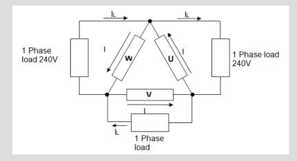
$I_{wdg} = I_L = 100A$  for each phase = 240V X 100A (1 phase) = 24kVA
