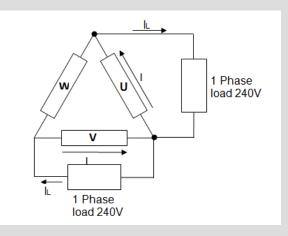
Each Single Phase load can be  $240V \times 100A = 24kVA$
