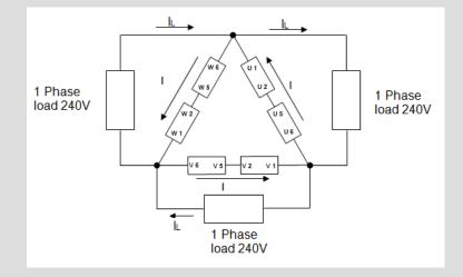
$I_{wdg} = I_L = 100A$  for each phase = 240V X 100A (1 phase) = 24kVA
