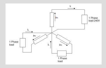
$I_{ph} = I_{L} = 100A$  for each phase = 240V x 100A (each phase) = 24kVA
