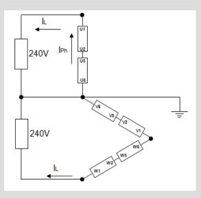
Supporting two individual single phase loads Each load =  $240V \times 100A = 24kVA$
