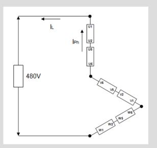
Supporting one individual 480V single phase load, because the effectively 1-Phase load is being 'driven' by a resultant voltage and therefore the load current is out of phase with the generated phase voltages, the  $I_L$  must be reduced to 75% of  $I_{wdg}$ .
