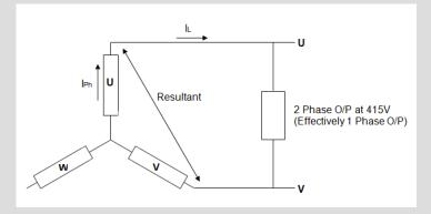
Because the effectively Single Phase load is being 'driven' by a resultant voltage and therefore, the load current is out of phase with the generated phase voltages, the  $I_L$  must be reduced to 75% of  $I_{Ph}$ . So,  $I_L$  will be 75A, Voltage will be 415V.
