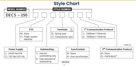
Compression type terminals are available for the current sensing (CT) inputs, operating power input, and power output connections only.
