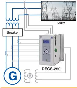
Figure 1 - DECS-250 Connection Diagram for a Typical Application
