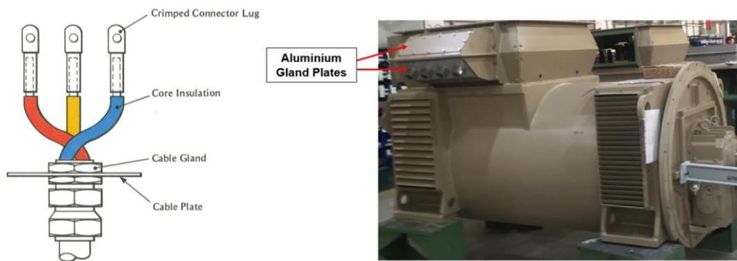
Figure 5: Showing an aluminium cable gland plates.
