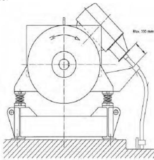
Figure 4: Showing a vibration damper for cable on the Generating Set foundation during installation.
