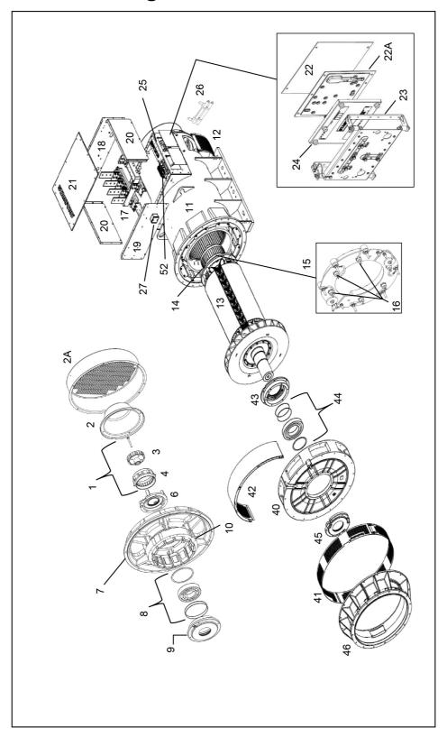
FIGURE 27. S7 TWO BEARING ALTERNATOR
