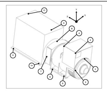
FIGURE 18. VIBRATION MEASUREMENT LOCATIONS
