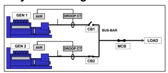
FIGURE 23. PARALLEL OR SYNCHRONIZING ALTERNATORS
