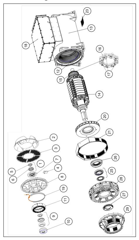
FIGURE 27. S9 TWO BEARING ALTERNATOR
