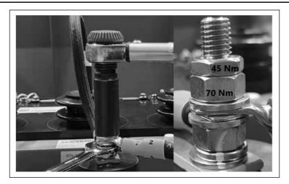
FIGURE 21. CORRECT CABLE CLAMPING (MULTIPLE CABLES)
