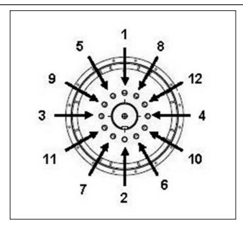
FIGURE 18. FIXING SEQUENCE TO HUB
