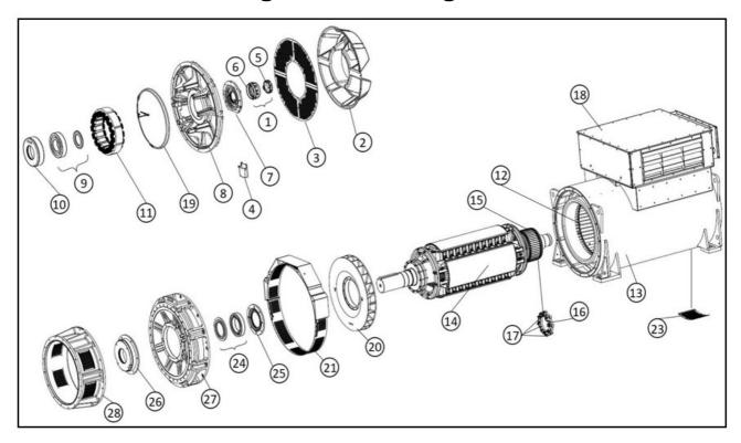
FIGURE 31. S9 LOW VOLTAGE TWO BEARING ALTERNATOR
