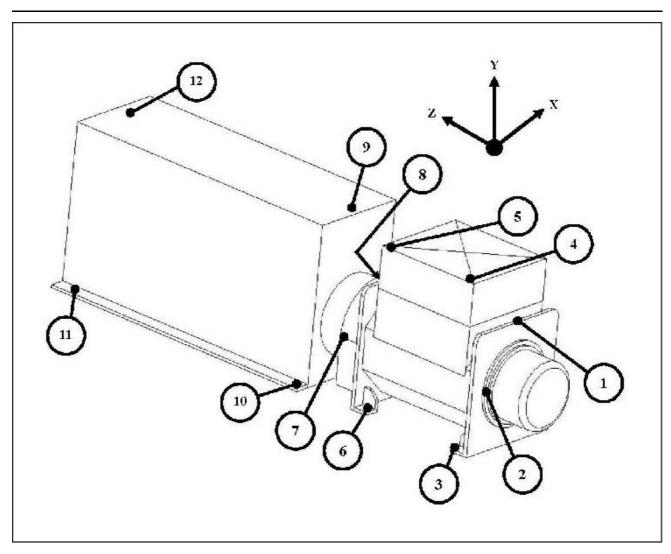
FIGURE 18. VIBRATION MEASUREMENT POSITIONS
