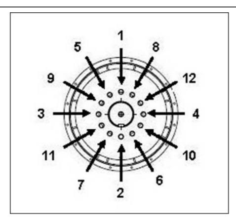
FIGURE 22. FIXING SEQUENCE TO HUB
