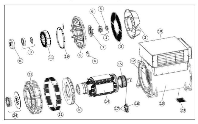
FIGURE 30. S9 LOW VOLTAGE ONE BEARING ALTERNATOR
