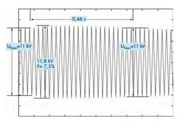
FIGURE 17. GENERATOR DIG 150I/8; 3300 KVA; 11 KV; 50 HZ; 750 MIN-1 SHUTTING DOWN 1000 KVA; COS  $\omega$  = 0.1
