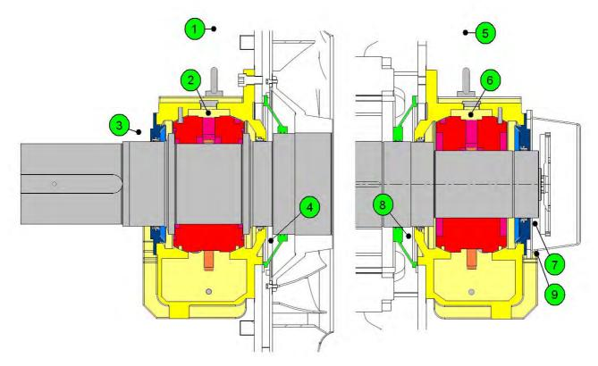
FIGURE 24. CHECKING THE AIR PRESSURE INSIDE AND OUTSIDE THE SLEEVE BEARING (1 - SLEEVE BEARING COVER)
