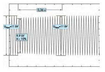
FIGURE 16. GENERATOR DIG 150I/8; 3300 KVA; 11 KV; 50 HZ; 750 MIN-1 SWITCHING IN 1000 KVA; COS  $\omega$  = 0.1
