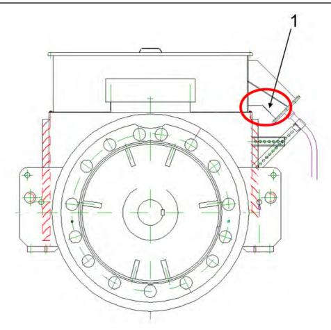
FIGURE 19. PROTECTION DEVICE (1)
