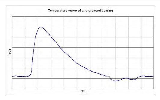
FIGURE 22. TEMPERATURE CURVE DURING RE-LUBRICATION
