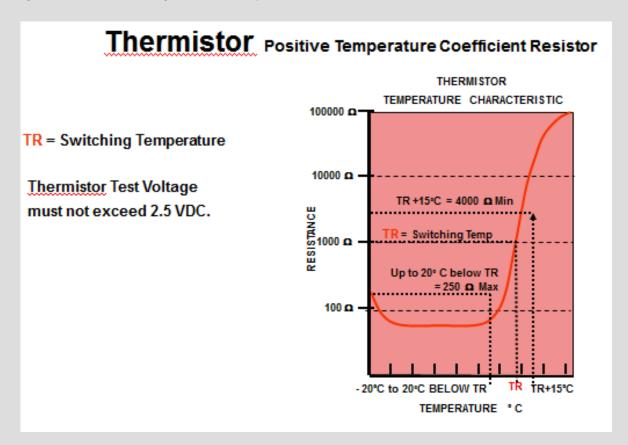
Typically, two of the above described thermistor schemes are incorporated, a system which operates at just above expected normal rated operating conditions and this scheme activates a control system function for triggering an ALARM.
