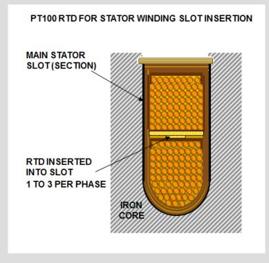
An alternators' winding temperature will be directly related to the kVA and power factor of the load, and so assuming an ambient of typically 30degC, an alternator will have 'roughly' the following component temperatures.
