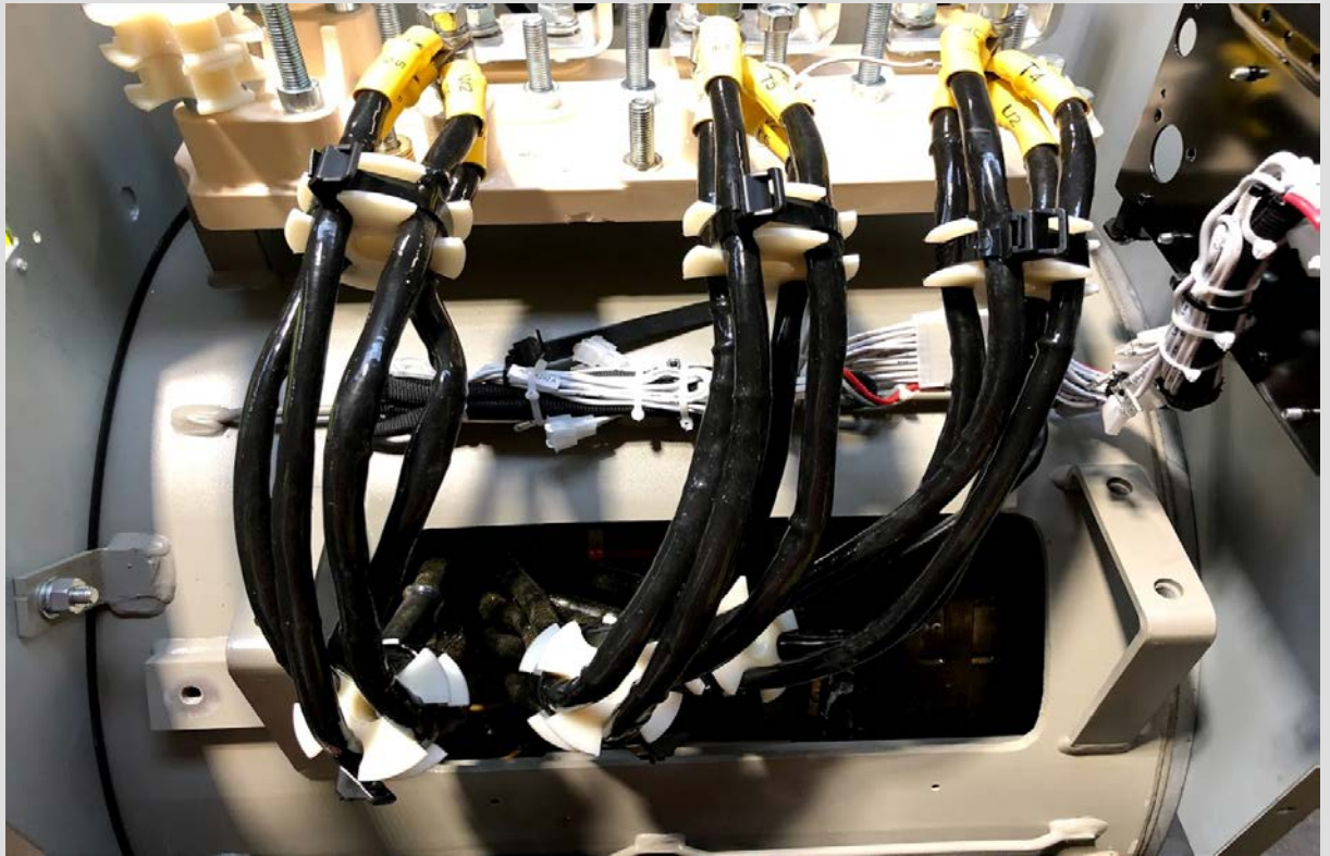
Figure 2: Stator Lead Spacers fitted to the S5L1D-G and S5L1D-H alternators.
