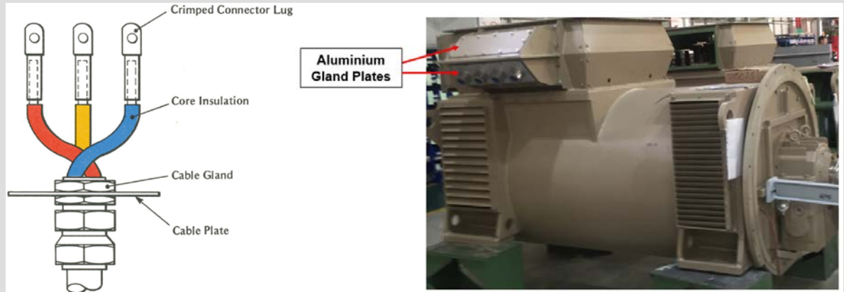
Figure 5: Showing an aluminium cable gland plates.
