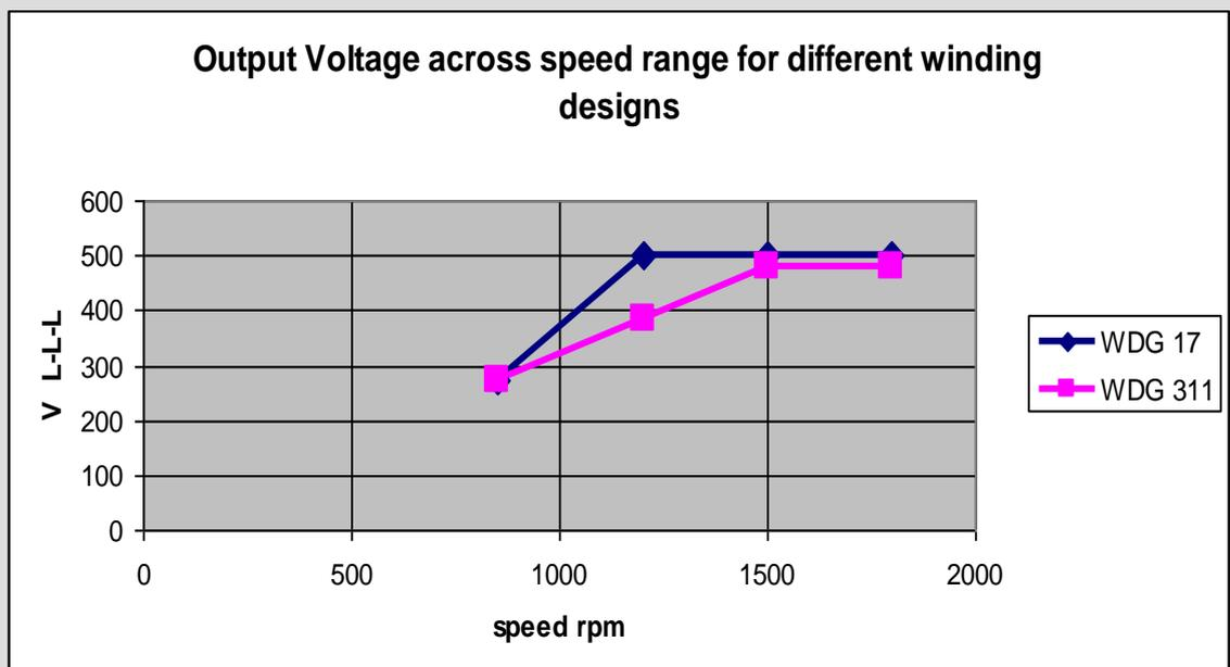
The graph on the previous page indicates a way forward for a fixed voltage across a speed range application. It indicates that over the 1200rpm to 1800rpm speed range, a constant voltage is possible. The technical explanations in preceding parts of this document have explained how the excitation system will be used to adjust the level of operational magnetic flux in order to maintain a constant voltage over a speed range.
