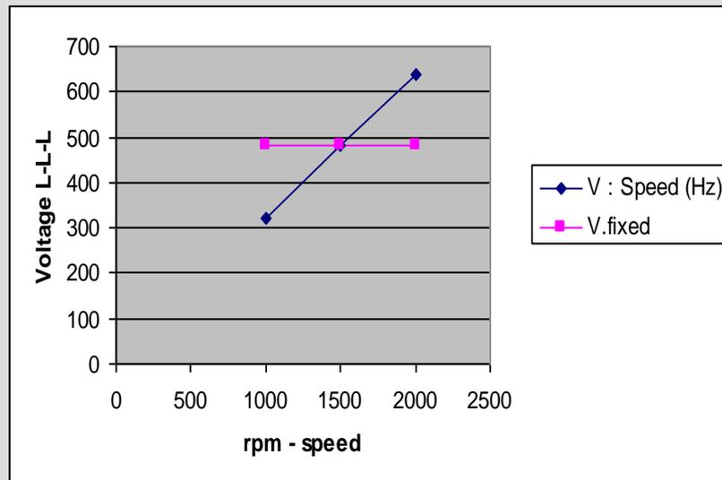
The 'Blue (diagonal) line' shows the ideal flux level being maintained when output voltage is proportional to speed. The 'Pink (horizontal) line' indicates a fixed voltage across the speed range.
