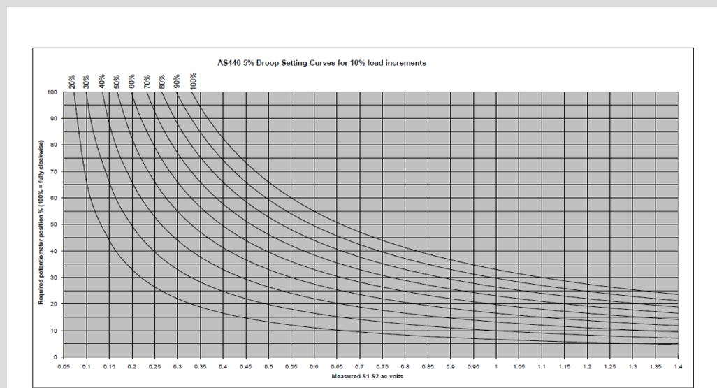
Figure 4: AS440 droop setting curves at various load
