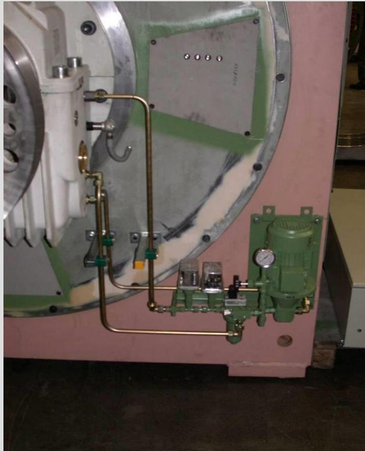
Hydrostatic jacking needs external oil flow and a considerable pressure in order to create a sufficient oil film which can carry the bearing load. Hydrostatic jacking is effectively used to minimize:
