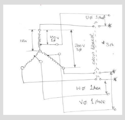
With the upgrade of alternators in the STAMFORD range, it has been decided to obsolete Winding 77. The outputs required for the Japanese national electrical distribution system, can now be supplied from STAMFORD alternators with the standard Winding 311, with a Parallel Star configuration.
