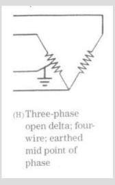
Note: the Code H configuration shows an open-delta, however; an AvK or STAMFORD alternator would always be connected in a full delta configuration.
