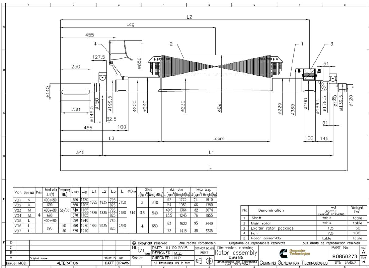
Figure 8: Typical alternator rotor drawing with shaft details.
