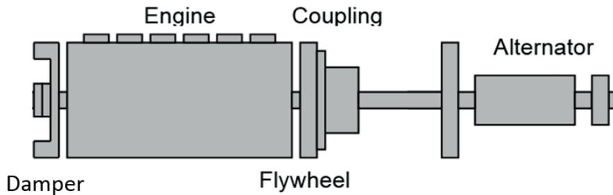
Figure 52: A complete Generating Set and areas for which data is required for TVA analysis.
