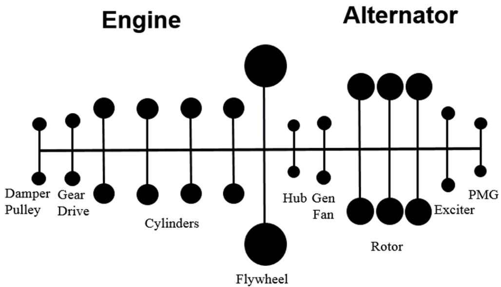
Figure 4: A complete Generating Set mass-elastic model.
