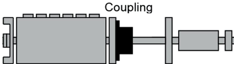
Figure 9: Coupling location for TVA analysis.
