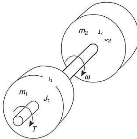
Figure 11: Two-mass torsional system.
