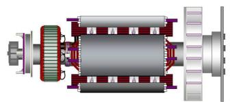
FIGURE 22. ONE BEARING ALTERNATOR ROTOR SHOWING COUPLING DISCS BOLTED TO DRIVE END COUPLING HUB (AT RIGHT)
