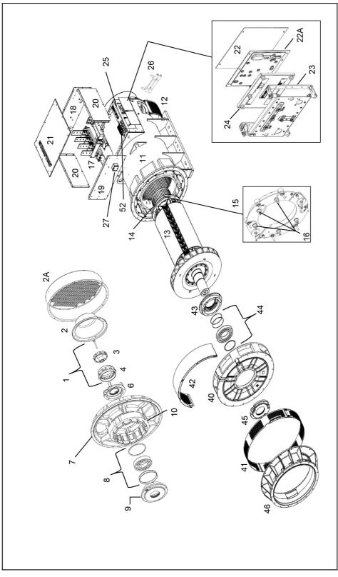
FIGURE 29. S7 TWO BEARING ALTERNATOR
