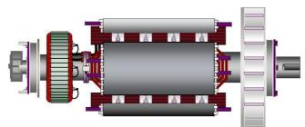
FIGURE 23. TWO BEARING ALTERNATOR ROTOR SHOWING SHAFT WITH KEYWAY FOR FLEXIBLE COUPLING (AT RIGHT)
