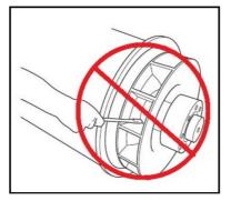
FIGURE 26. DO NOT ROTATE THE ALTERNATOR ROTOR WITH A LEVER
