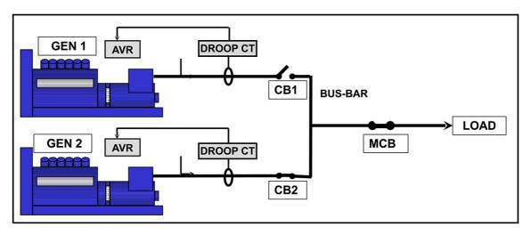
FIGURE 25. PARALLEL OR SYNCHRONIZING ALTERNATORS
