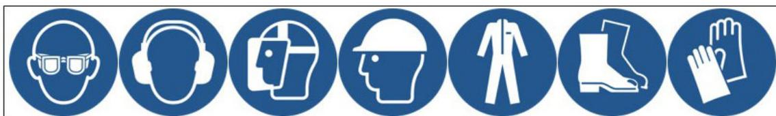
FIGURE 1. ÉQUIPEMENT DE PROTECTION PERSONNELLE (PPE) MINIMUM RECOMMANDÉ
