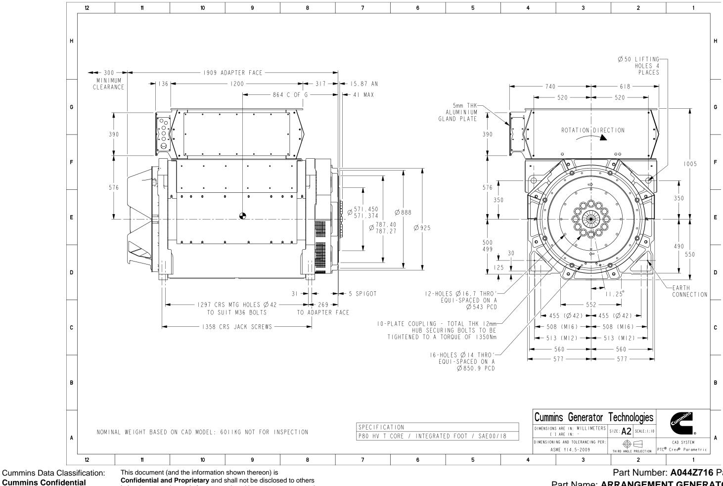
**Confidential and Proprietary** and shall not be disclosed to others in hard copy or electronic form, reproduced by any means, or used for any purpose without written consent of Cummins Inc. Part Number: A044Z716 Part Revision: B Part Name: ARRANGEMENT,GENERATOR GENERAL Drawing Category: Outline (Tabulation) State: Released Sheet 1 of 3
