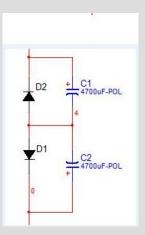
Figure 3: Capacitor-diode circuit diagram for droop CT polarity check
