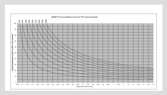
Figure 4: AS440 droop setting curves at various load
