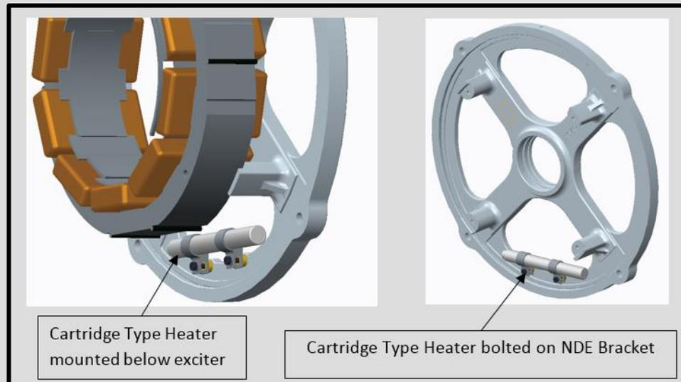
Heater options for the S1L2 are (Drawing A12-H11):
