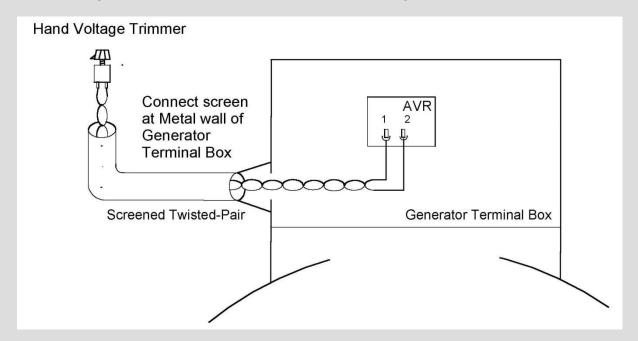
The suggested cable specification for this example is: 0.75mm2, 3A/500Vac minimum screened and jacketed twisted-pair.
