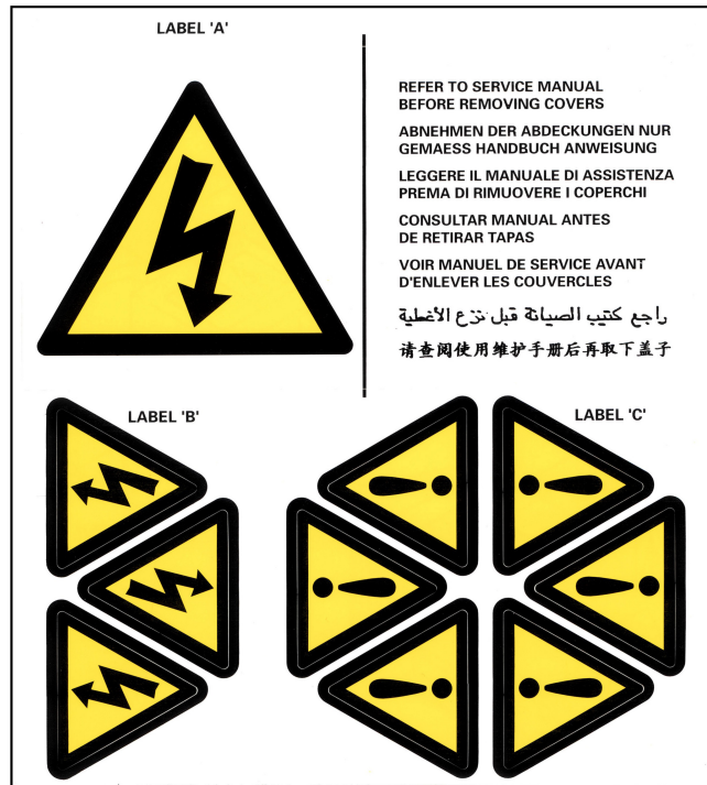
FIGURE 2. HAZARD WARNING LABELS
