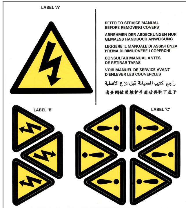
FIGURE 2. HAZARD WARNING LABELS
