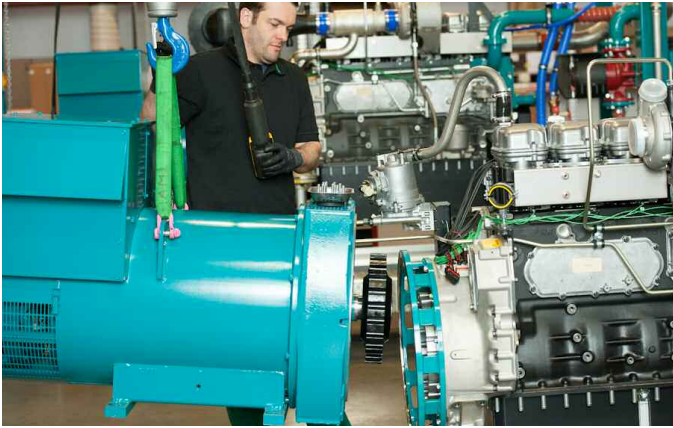
Coupling the STAMFORD ® alternator to the engine at SCHNELL'S headquarters in Amtzell, Germany
