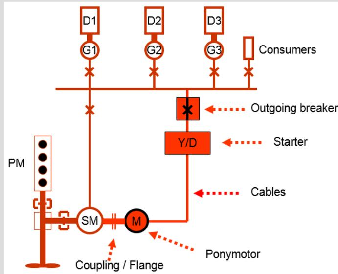
The starter for the pony motor could be Star/Delta, Electronic Soft Starter, Autotransformer or Inverter/VFD, fed by the auxiliary generators G1, G2, G3 as shown.
