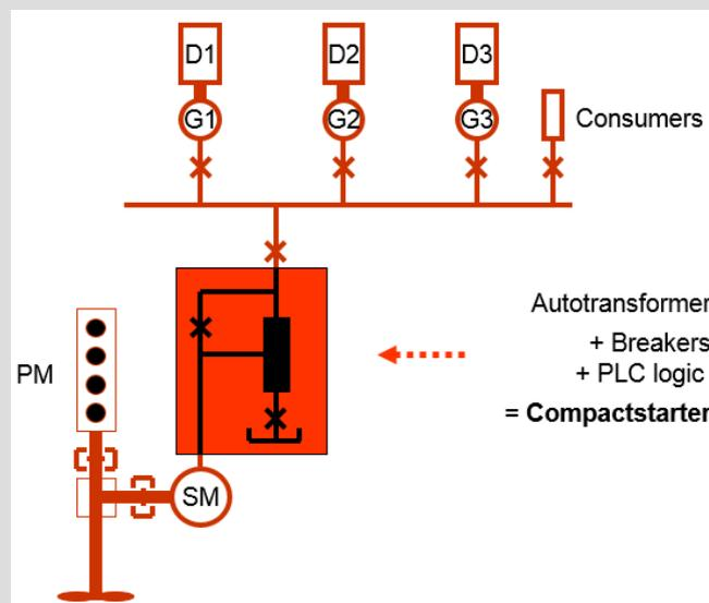
The shaft generator is started as an asynchronous motor with this method and therefore, requires some modifications to the excitation system of the machine. These modifications are explained later on in this AGN.
