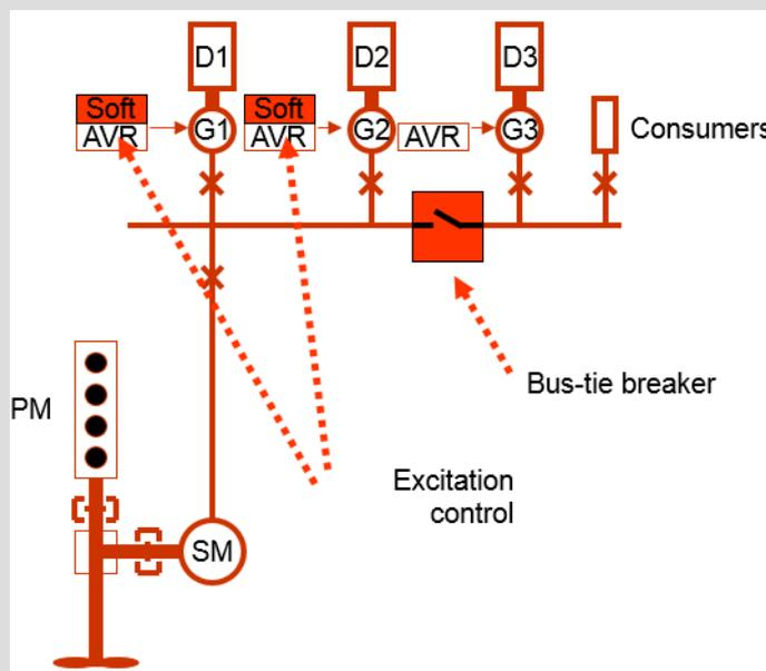
As with the Auto-Transformer Start described in Option 2, the machine is started asynchronously and so requires some excitation system modifications.
