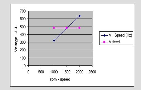
The 'Blue (diagonal) line' shows the ideal flux level being maintained when output voltage is proportional to speed. The 'Pink (horizontal) line' indicates a fixed voltage across the speed range.
