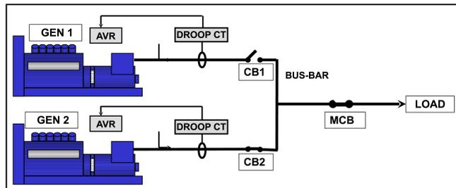
**FIGURE 22. PARALLEL OR SYNCHRONIZING ALTERNATORS**
