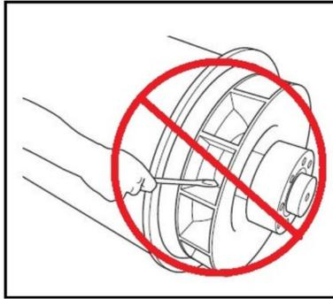
**FIGURE 14. DO NOT ROTATE WITH A LEVER**
