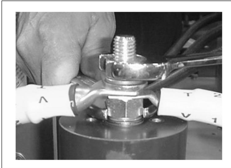
**FIGURE 20. CORRECT CABLE CLAMPING (MULTIPLE CABLES)**
