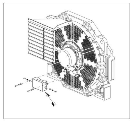
FIGURE 23. GREASE TRAP ON P80 ALTERNATORS WITH AN AIR FILTER
