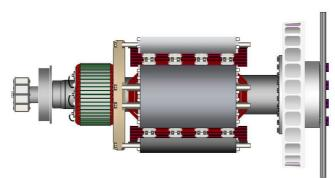
FIGURE 15. SINGLE BEARING ALTERNATOR ROTOR SHOWING COUPLING DISCS BOLTED TO DRIVE END COUPLING HUB (AT RIGHT)
