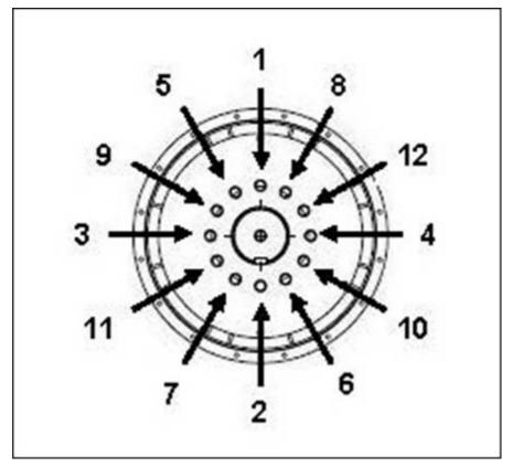
FIGURE 17. FIXING SEQUENCE TO HUB
