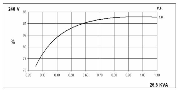
PM144G Winding 06 Locked Rotor Motor Starting Curve
