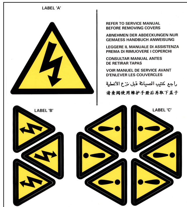
FIGURE 2. HAZARD WARNING LABELS
